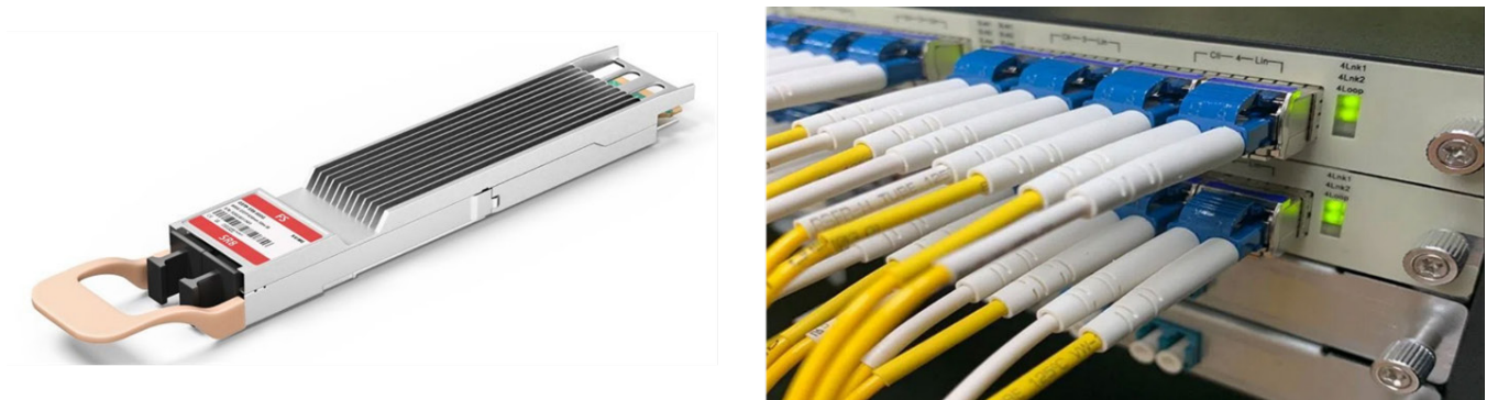
Figure 1. The left shows a pluggable optical transceiver (from FS.com). The finned end of the transceiver gets plugged into a switch and the black caps on the opposite end are removed to plug in optical fibers. The right shows a switch full of pluggable optical transceivers (from Unitekfiber.com).
